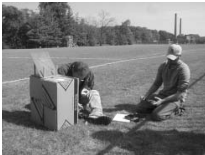
Figure 1. A pedestal with board for inclination measurement set up on the soccer field of Ball State University. We encourage students to work in small groups but require that everybody reports their own measurements.
